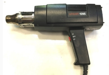
Fig. 8: Heat gun for shrink wrap insulation
