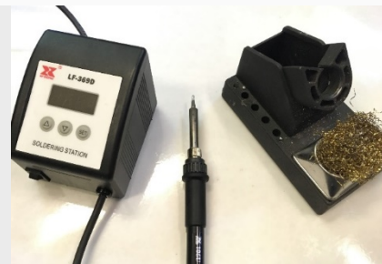
Fig. 9: Temperature-controlled soldering iron/station
