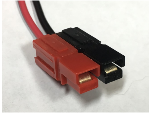
Fig. 31: Proper orientation of housing
